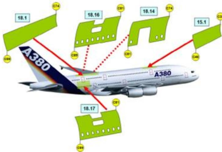
Figure 1: GLARE fuselage panels made by Tier-1-Supplier PAG in Nordenham /Germany [a]
