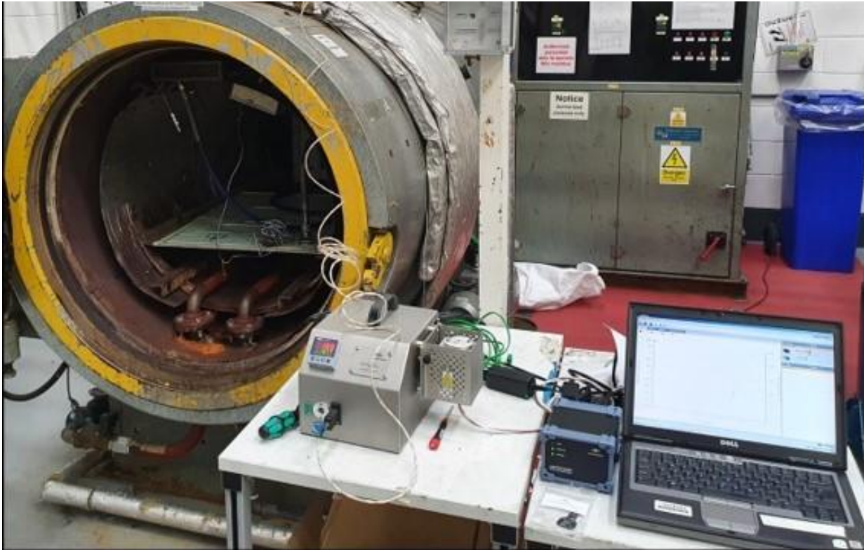
Left: The Cure Simulator system at the R&D autoclave at NIACE, Belfast, Right: The flat mould with the preform installed in the autoclave.
