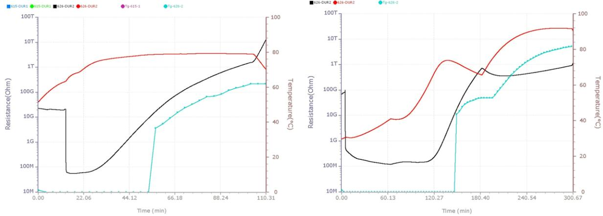
**Figure 9:** Typical ORS graphs showing the resistance (left vertical axis) together with temperature and  $T_g$  (right vertical axis). Left figure: Isothermal case, Right figure: Strongly non-isothermal case
