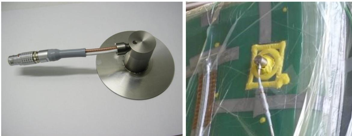
**Figure 7:** Left: The new durable vacuum bag sensor; Right: Installed at production
