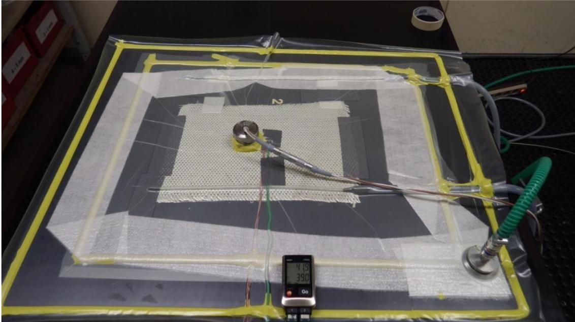
**Figure 8:** A typical vacuum infusion set-up of a laminate together with cure and temperature sensors on top of the vacuum bag.
