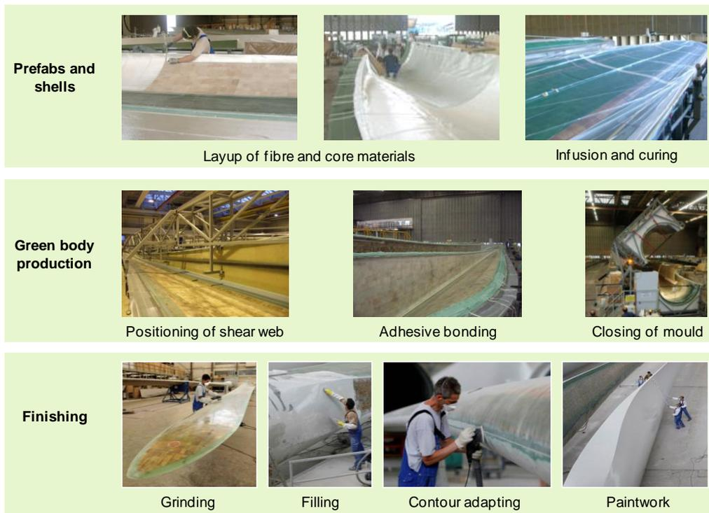
**Figure 6:** Production steps for rotor blades
