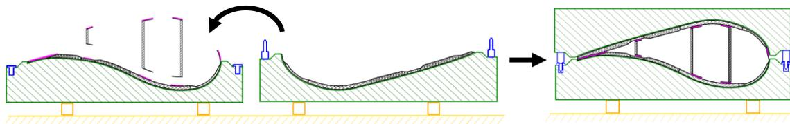
**Figure 3:** Widespread production method for rotor blades
